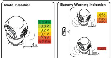
**Warning Indication.** In ON-state shows the battery voltage and the temperature inside the headlamp.
