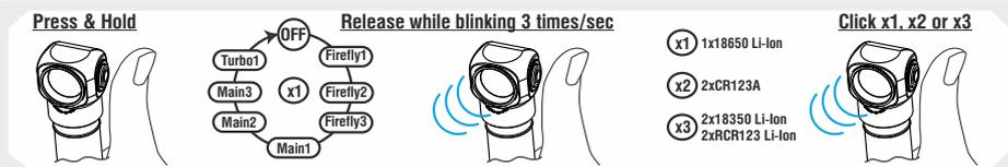
To access the Menu press and hold the switch button (when the flashlight is switched off). It will switch on, go through 7 modes, then after 2sec in Turbo1 mode – enter to Menu and flash about 3 times a second.
